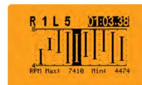
Min/Max RPM per lap
